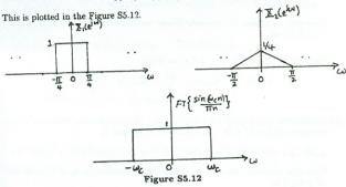
From Figure S5.12 it is clear that  $X_2(e^{i\omega})$  is zero for  $|\omega| > \pi/2$ . By using the convolution property (Table 5.1, Property 5.4), we note that
