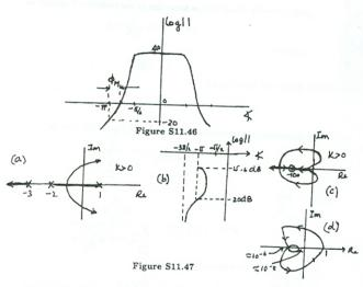
For the gain margin, we first need to find  $\omega_0$  such that  $\langle G(j\omega_0)H(j\omega_0) = -\pi$ . For this we need  $\omega_0 = 93$ . Now,  $|G(j\omega_0)H(j\omega_0)| = -24.7$  dB. Therefore the gain margin is 24.7 dB.
