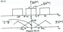
From the figure, it is clear that we require  $-1+(2\omega_c/\pi)$  to be 1/2. Therefore,  $\omega_c=3\pi/4$ .
