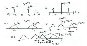
8.47. Let  $G_c(e^{j\omega})$  represent the Fourier transform of  $\cos(\omega_c n + \theta_c)$ . This is as shown in Figure S8.47. Let  $G_d(e^{j\omega})$  represent the Fourier transform of  $\cos(\omega_d n + \theta_d)$ . This is as shown in Figure S8.47.
