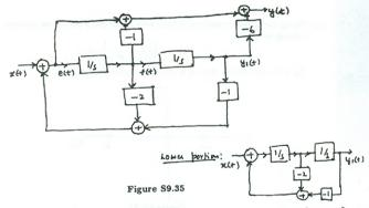
Therefore,  $f(t) = dy_1(t)/dt$ . Similarly, e(t) = df(t)/dt. Therefore,  $e(t) = d^2y_1(t)/dt^2$ . From the block diagram it is clear that
