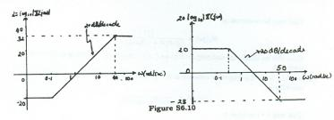
(b) Using a similar approach as in part (a), we obtain the Bode plot to be as shown in Figure S6.10.
