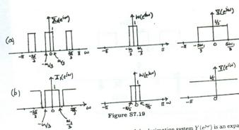
The Fourier transform of the output of the decimation system  $Y(e^{j\omega})$  is an expe or stretched out version of  $W(e^{j\omega})$ . This is as shown in Figure S7.19. Therefore,
