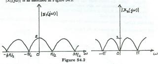
(a) The signal  $x_1(t) = \sin(2\pi t + \pi/4)$  is periodic with a fundamental period of T = 1. This translates to a fundamental frequency of  $\omega_0 = 2\pi$ . The nonzero Fourier series coefficients of this signal may be found by writing it in the form
