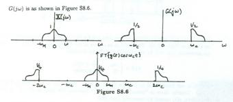
The Fourier transform of  $g(t)\cos(\omega_c t)$  is also shown in Figure S8.6. Clearly, if we want to recover x(t) from  $g(t)\cos(\omega_c t)$ , then we have to pass  $g(t)\cos(\omega_c t)$  through an ideal lowpass filter with gain 4 and cutoff frequency  $\omega_M$ . Therefore, A=4.
