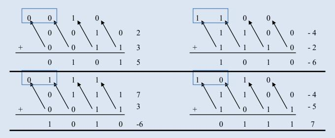
So how do we detect overflow for signed arithmetic?
