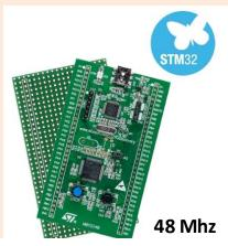
The Cortex-M0 processor is built on a highly area and power optimized 32-bit processor core, with a 3-stage pipeline von Neumann architecture. The processor delivers exceptional energy efficiency through a small but powerful instruction set and extensively optimized design, providing high-end processing hardware including a single-cycle multiplier.
