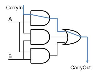
The point: ripple carry adders are slow. Faster addition schemes are possible that *accelerate* the movement of the carry from one end to the other. Optimizing this is *digital logic* (CSE 140).
